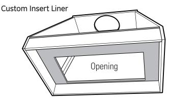
The custom canopy must be sized to fit the insert sleeve. Construct the canopy with an opening that is: 38-3/4"W x 13-3/16"D
